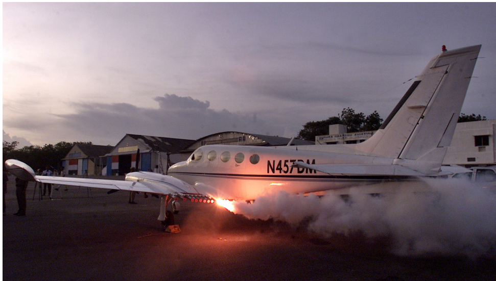
Cloud seeding flares mounted on an aircraft [Source]
